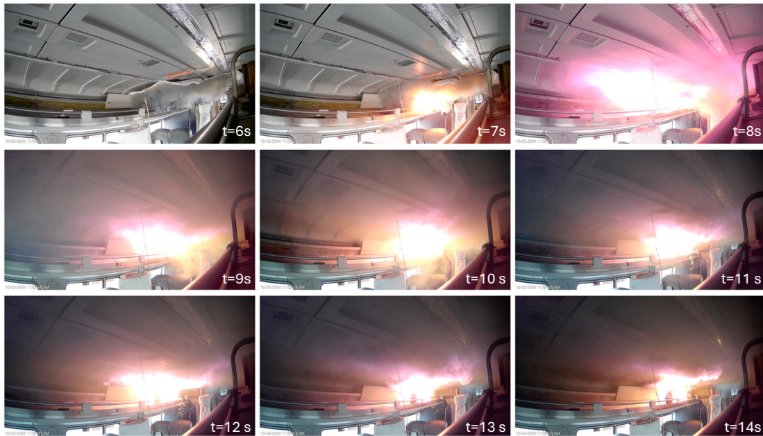
Figure 5 – Video sequence from the standing e-scooter experiment, video sequence starts 1 s before ignition of the battery gas, images are shown at 1s intervals, t=0 s is at ignition.
