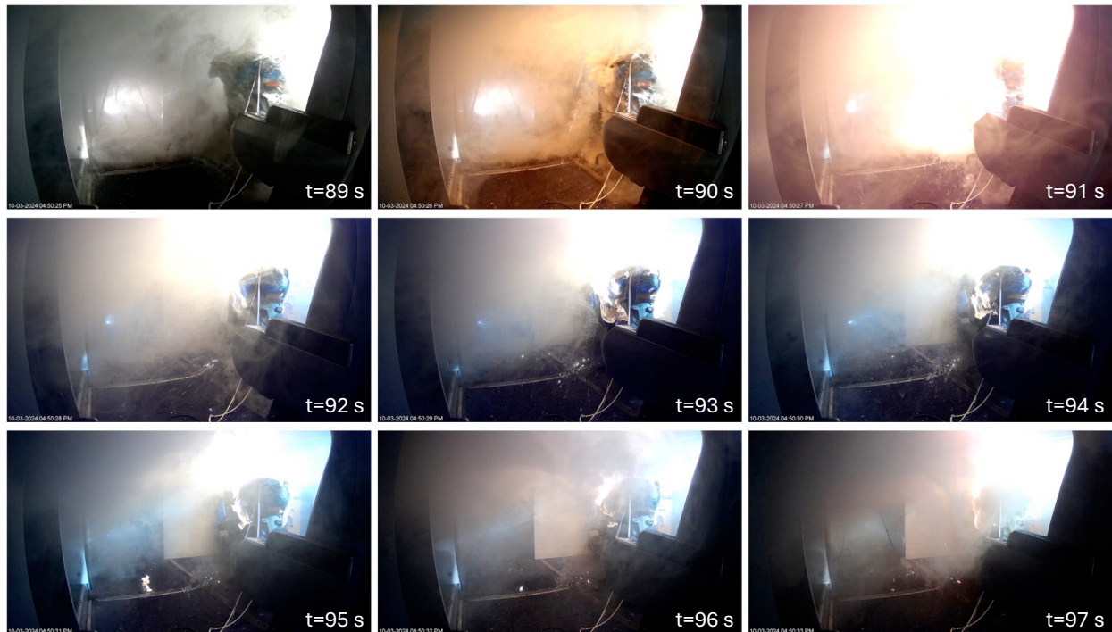
Figure 7 – Video sequence for the first seated e-scooter experiment starting 1 s before ignition of the battery runaway gases were visible, images are shown at 1 s intervals, t=90 s at ignition.
