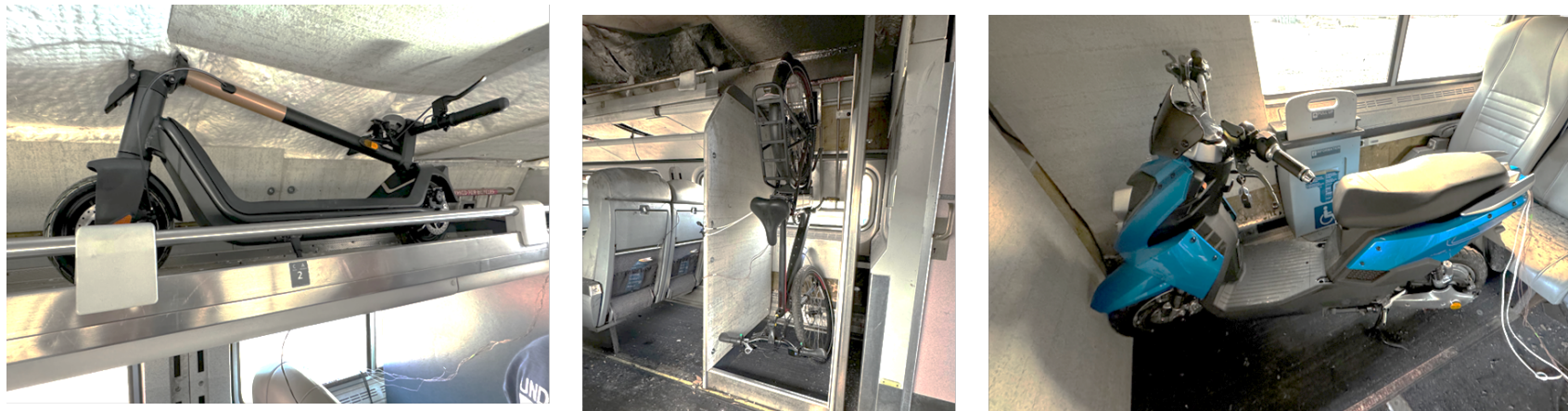
Figure 3 - Photograph of the standing e-scooter (left), e-bicycle (center) and seated e-scooters (right), in situ just prior to starting ignition.
